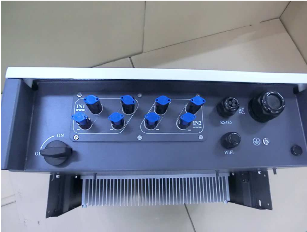
Terminals view of the unit for model Sofar 10000TL-Sx
