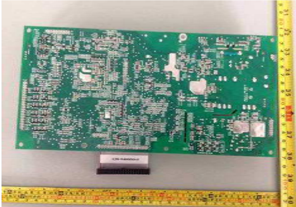
Bottom view of the control board
